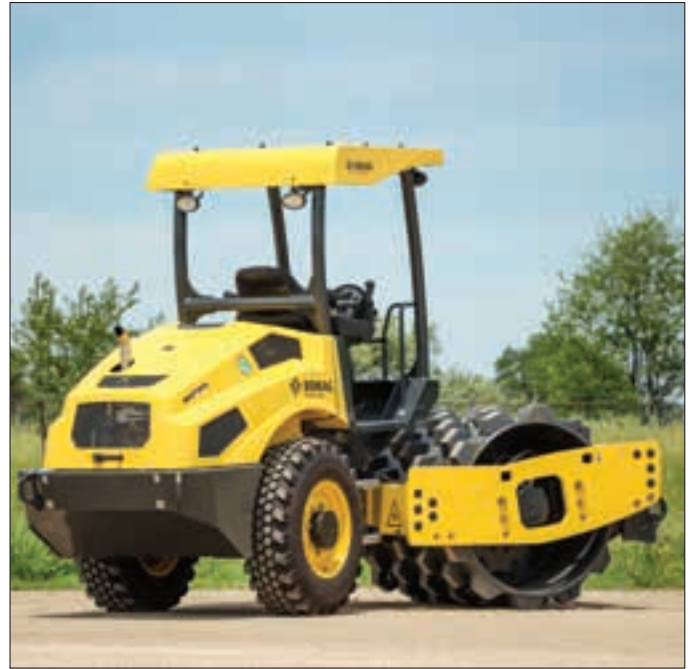
Operator's cockpit features dual entry accessibility.
